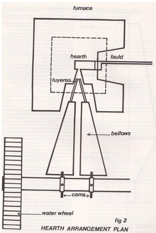
The hearth's vertical walls met the bottom of the bosh some 2 ft. or more above the bottom stone. The bosh extended up the furnace for at least 4 ft. gradually widening until at the top of the bosh, the furnace reached its widest internal measurement; the early furnaces were about 6 ft. across at this point.
