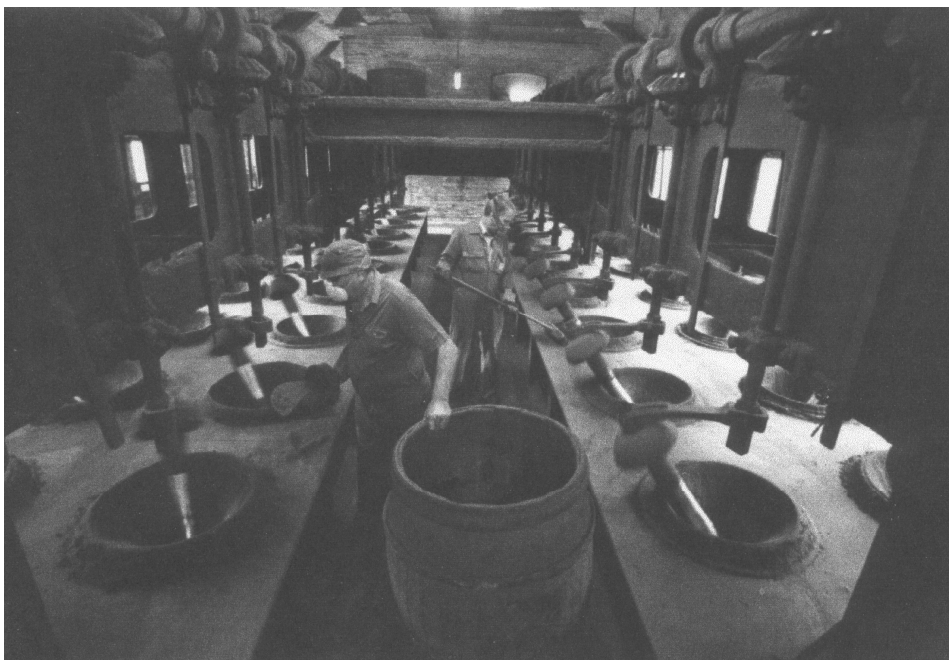
Plate 1 Lines of water-powered pestels and mortars at Sharrow snuff mill, Sheffield, c1990.
