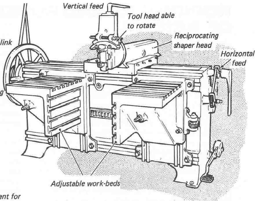
from the front of the machine between the two tables, is the rotating socket which can accept a shaft, called a mandrel, on which work can be mounted. The machine can thereby cause the tool to reciprocate above the mandrel, but parallel to its axis, whilst the mandrel is slowly rotated. It was thus possible to shape a cylindrical form, a facility which was used to produce splined bushes. (Splines are a form of teeth, placed around a shaft, which are parallel to its axis).
