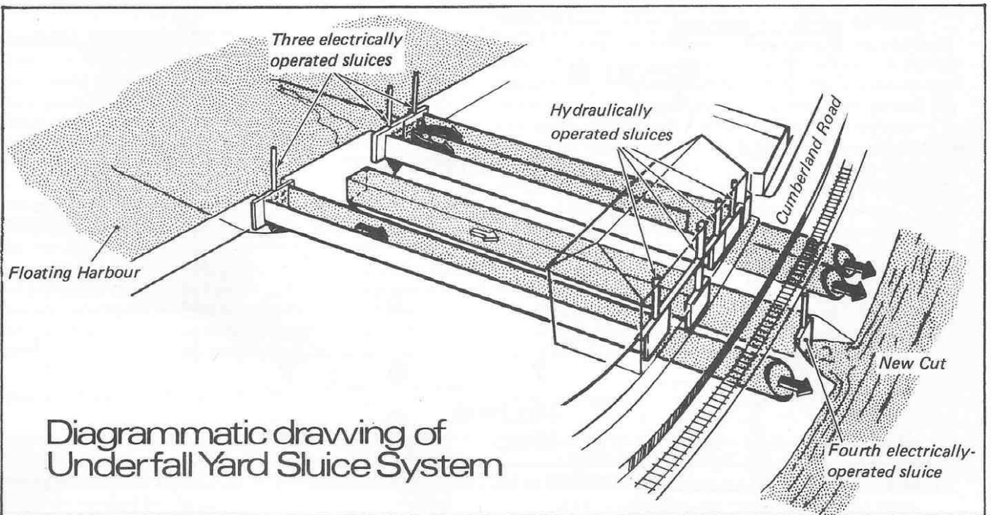
Diagrammatic drawing of Underfall Yard Sluice System
