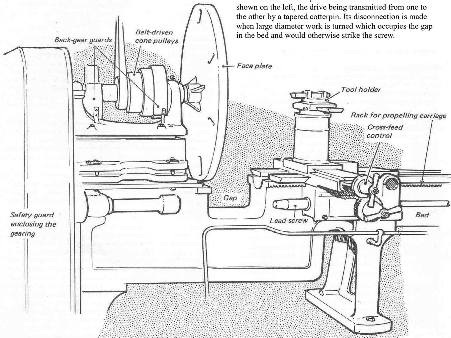
The drawing shows a horizontal bar in the foreground similar to a handrail in appearance. This, in fact, is a belt-striker control, extending just over halfway along the machine, and it eliminates the need for the return of the operator to the headstock each time a start or stop is required. Owing to the machine's length, this control is more than a convenience; it is an essential item.
