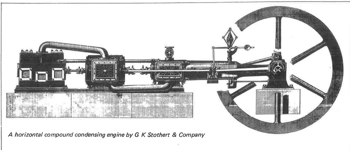
*A horizontal compound condensing engine by G K Stothert & Company*
