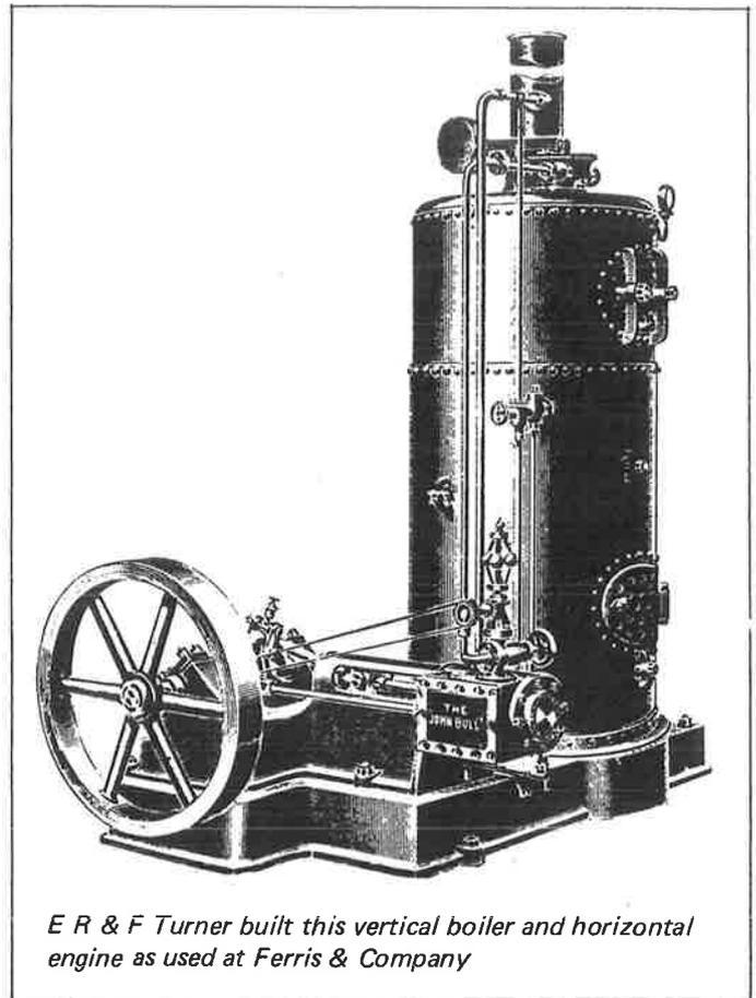
*E R & F Turner built this vertical boiler and horizontal engine as used at Ferris & Company*
