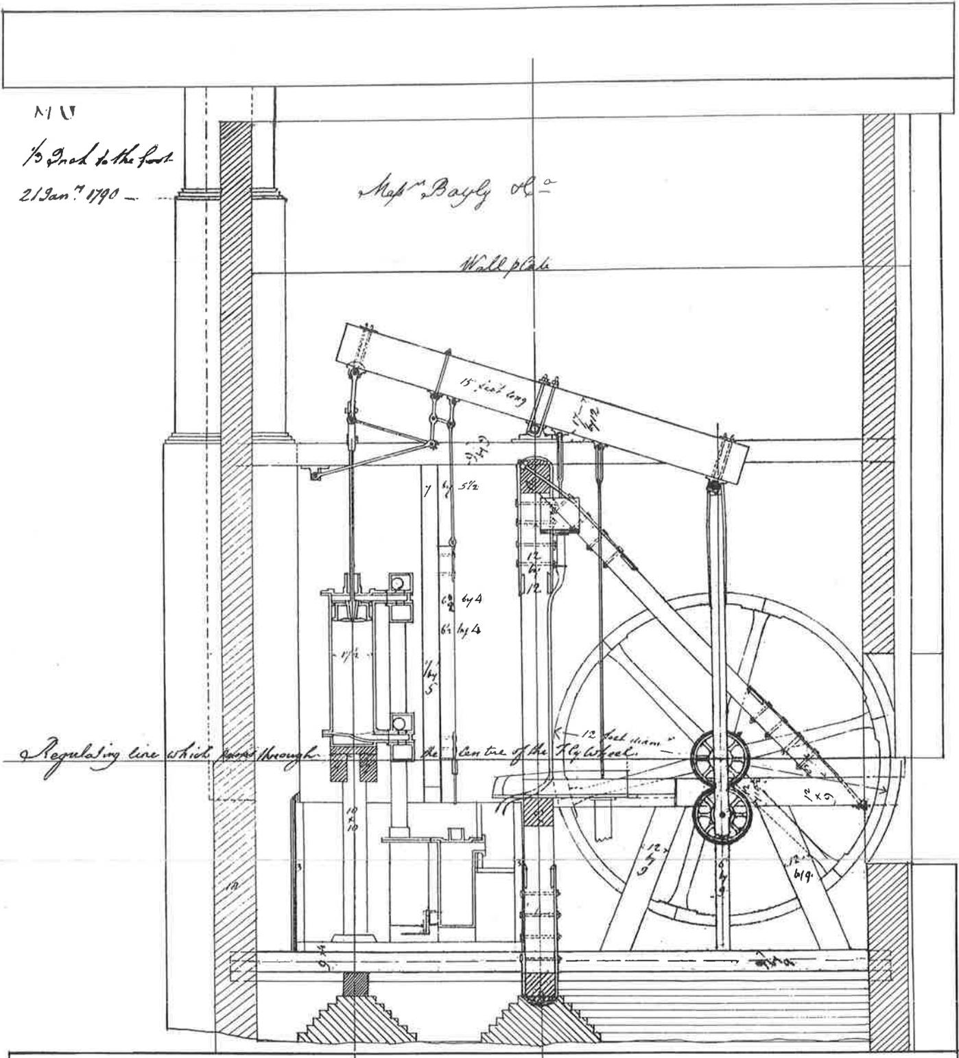
**Drawing of 10hp engine supplied by Boulton and Watt to the Lead Works of Robert Bayly and Company of Lawrence Hill in 1790**
