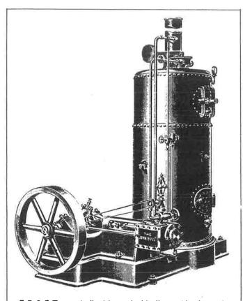
E R & F Turner built this vertical boiler and horizontal engine as used at Ferris & Company
