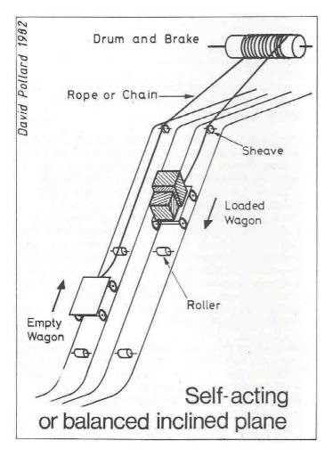
Bath stone railways made after the 1830s belong to the third phase of development, and were characterised by a uniform track gauge of 2 ft  $5\frac{1}{2}$  ins, wrought~iron and steel rails and by standardised rolling stock. These true narrow gauge railways were used both for internal quarry transport as well as carrying stone to the Great Western Railway.
