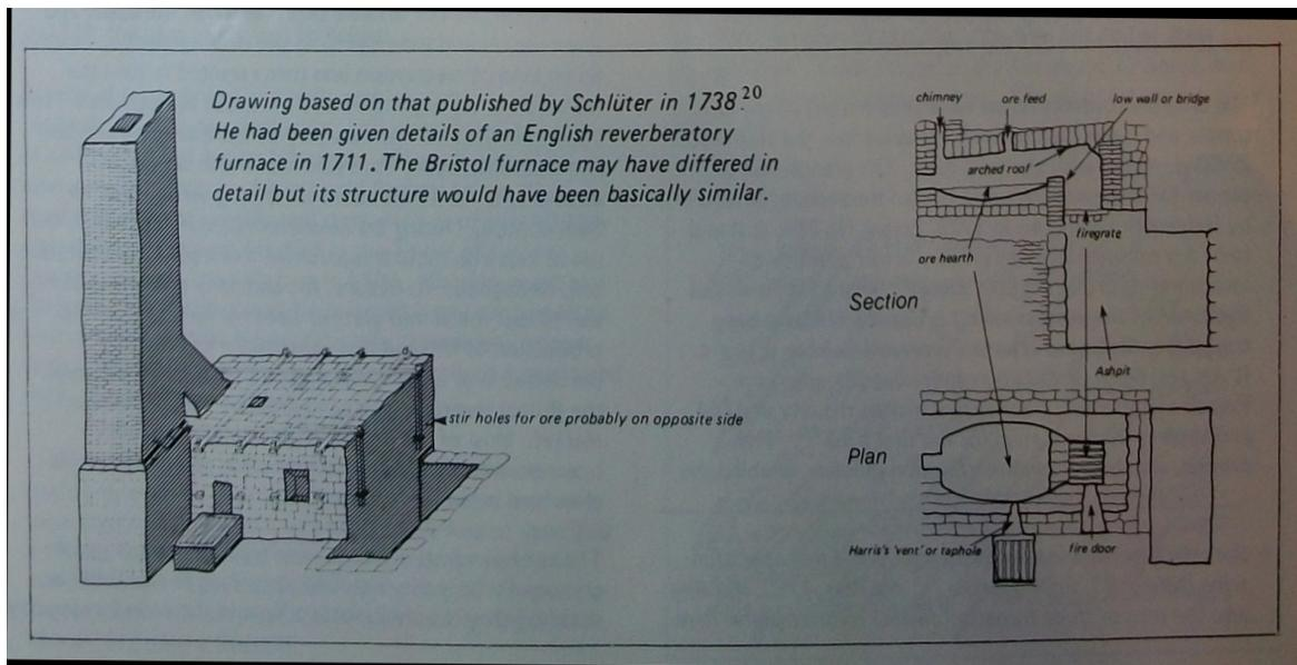
*Drawing based on that published by Schlüter in 1738<sup>20</sup>. He had been given details of an English reverberatory furnace in 1711. The Bristol furnace may have differed in detail but its structure would have been basically similar.*
