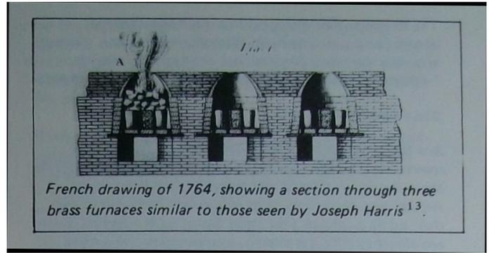
zinc vapour to permeate the greater surface area of the copper granules more efficiently. The furnace temperature, approaching 1000°C, was kept carefully below the melting point of copper to allow the granules to remain distributed throughout the mass in the crucible. Granulation improved the yield because less zinc vapour was wasted to the atmosphere.
