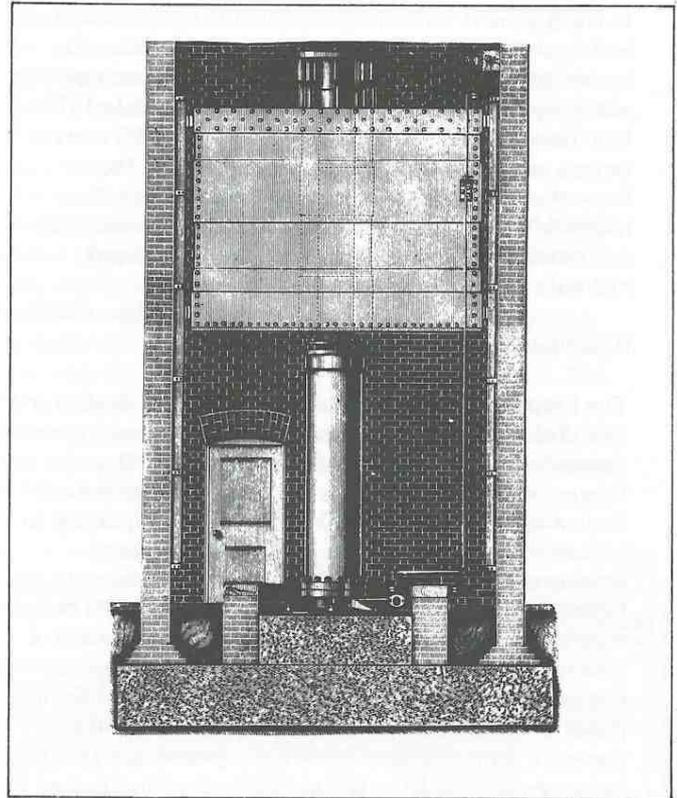
A typical arrangement of a hydraulic accumulator: in the late 19th century
