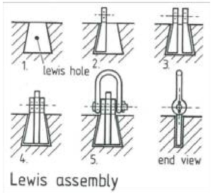
Lewis holes were started with picks and finished off with holing irons. What is remarkable is that this range of tools with the addition of a few others survived into recent times and co existed with power tools in partly mechanised quarries. Cranes were used at Combe Down from about 1730 and were common by 1812.
