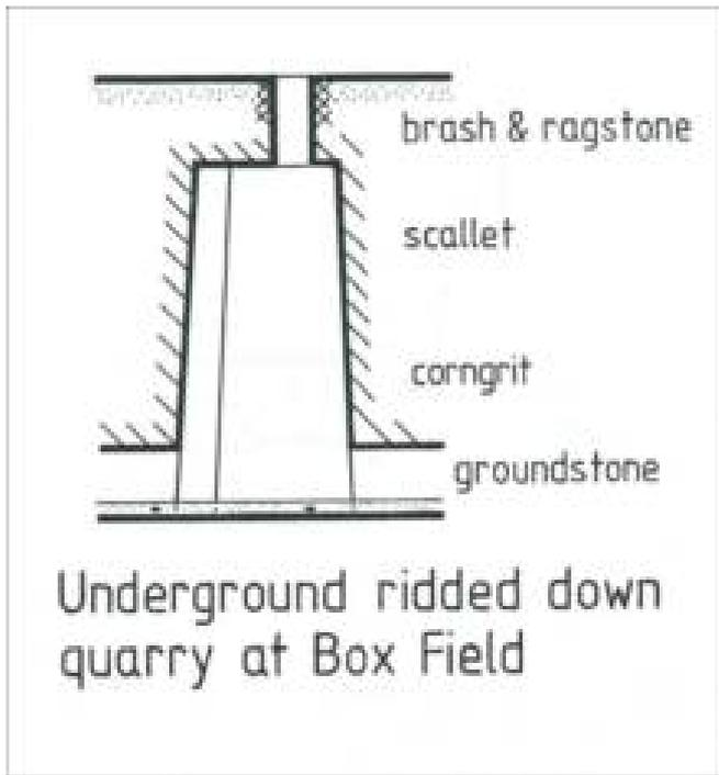
1908 to replace the existing vertical winding shaft <sup>(6)</sup>. Shaft haulage was by stationary steam engines, portable steam engines driving cable drums, ginny rings, twin cylinder single drum capstans, a Fowler ploughing engine and finally an electric winch.
