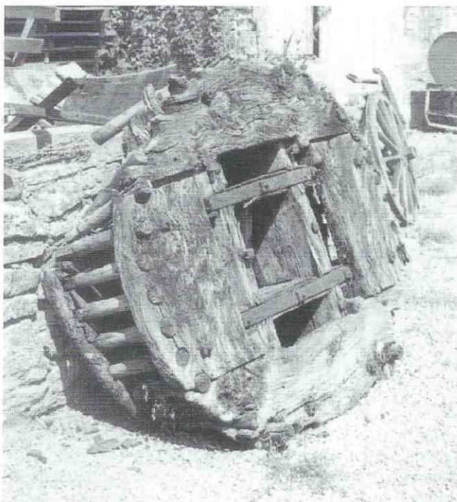
A decaying wooden gear from Powdermill
