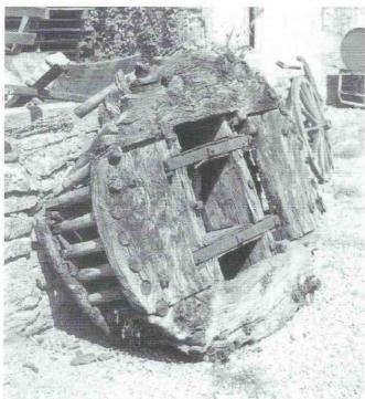
A decaying wooden gear from Powdermill
