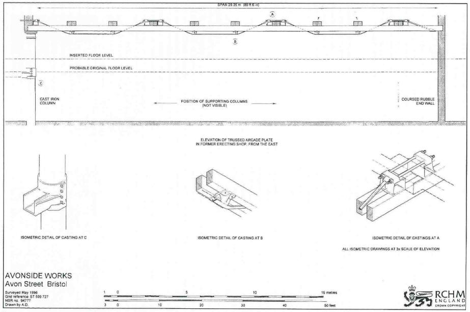
Fig 3 Elevation of the trussed arcade plate in the former erecting shop, from the east, and isometric details
