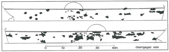
HMS Ruby: hull damage received 6-7 August 1846 from 40 shots fired by HMS Excellent.
