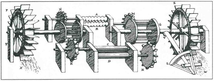
Fig 2 Diagram of a slitting mill
