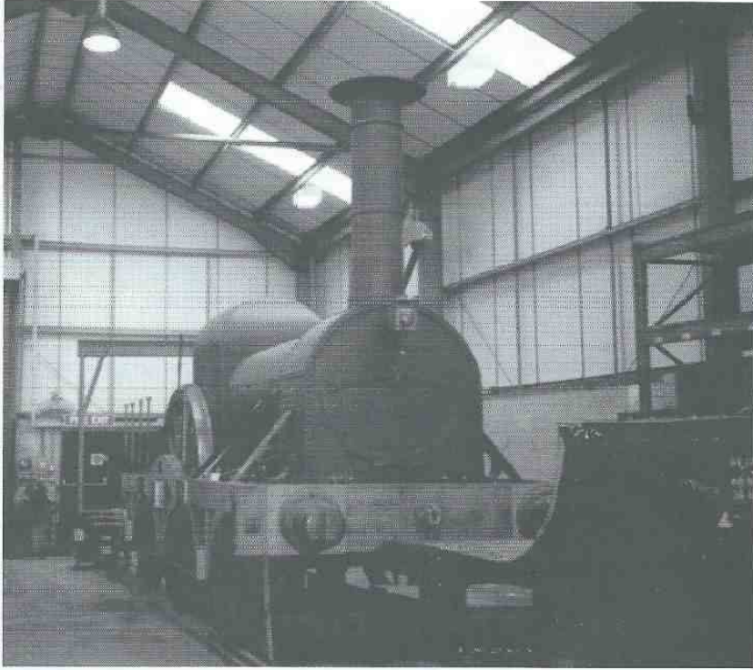
Smoke box and chimney backed by the dummy boiler and fire box
