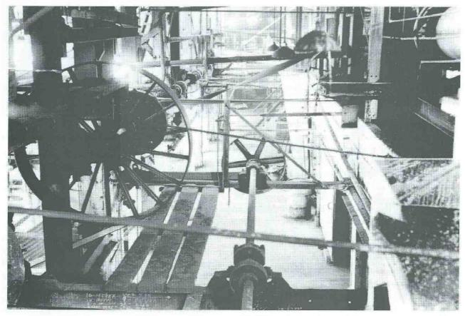
Line shafting and belt drives to machinery
